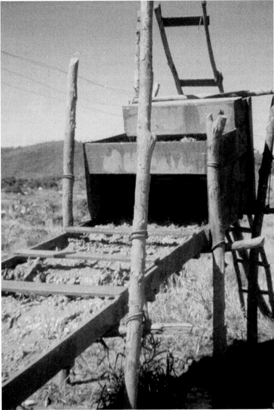
A cobra fumando used for underground mineshafts (of about 200 feet in depth). The pulp is suctioned by a pump, and goes through a system of wooden boxes for the recovery of gold. Photo: J. Graulau (2000).
